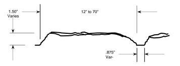
Standard sheet size: 48" x 360" (two formliners together) Interlocking pattern (Type-A—Type-B)
